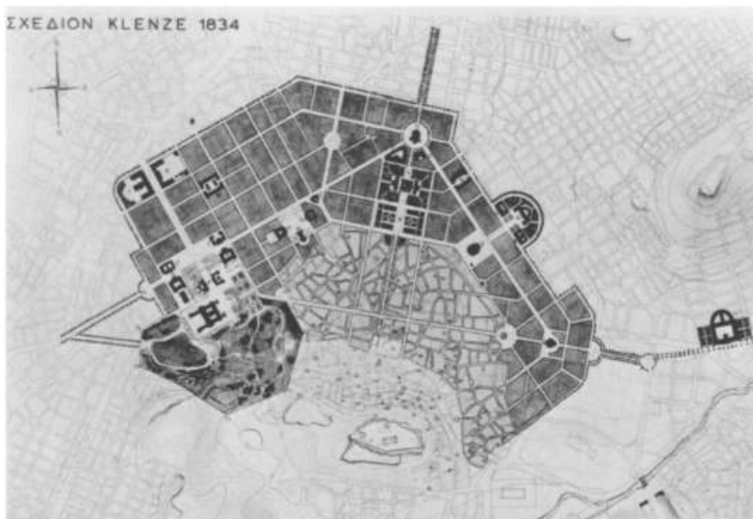
Figure 2.20 Klenze's master plan for Athens 1834. The three central axes can be seen passing through the traditional city. (Source: Thirlwall, 1846, p3.026)
